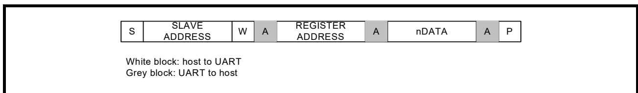
FIGURE 4. MASTER WRITES TO SLAVE (XR20M1170)
