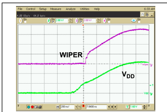
FIGURE 2-52: 50 k \Omega – Power-Up Wiper Response Time.
