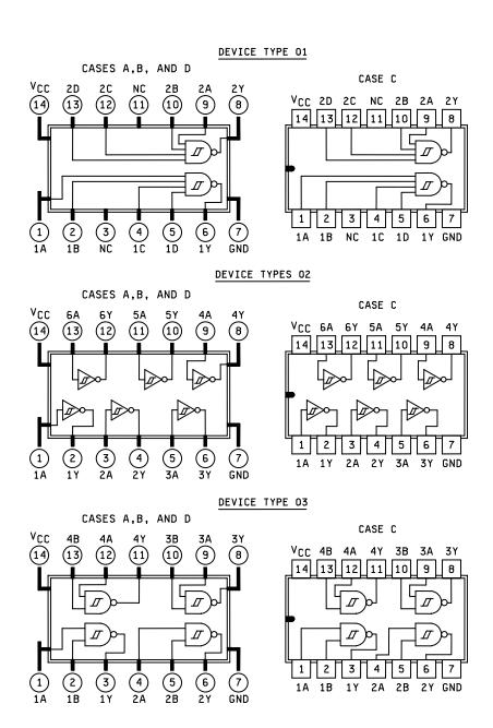
Figure 1. Logic diagrams and terminal connections (top view).
