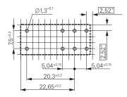
\*) With the recommended PCB hole sizes a grid pattern from 2.5mm to 2.54mm can be used
