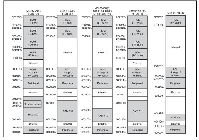
Note : The high-order portion of bank 00 gives the image of the FF bank ROM to make the small model of the C compiler effective. Since the low-order 16 bits address are the same, the table in ROM can be referenced without using the "far" specification in the pointer declaration.
