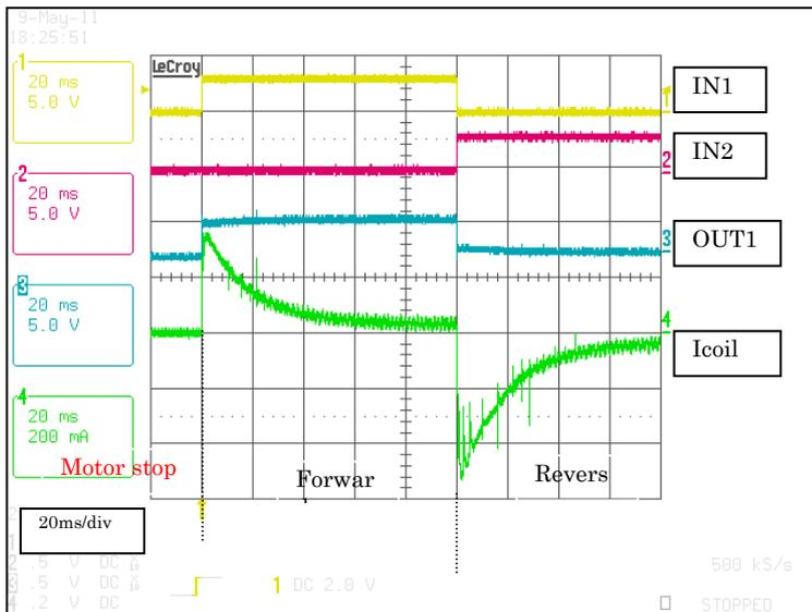
If a direction of rotation is switched while the DC motor is under rotation, torque for reverse rotation is generated. Therefore, the change of rotation takes place more abruptly.
