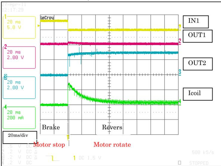
High current flows when the DC motor starts to rotate. After a while, induced voltage "Ea" is generated from motor and current value gradually decreases in the course of motor rotation.
