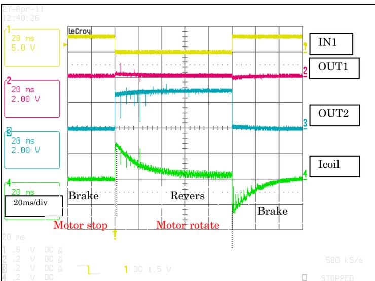
By setting brake mode while the DC motor is under rotation, DC motor becomes short-brake state and thereby decreases rotation count rapidly.
