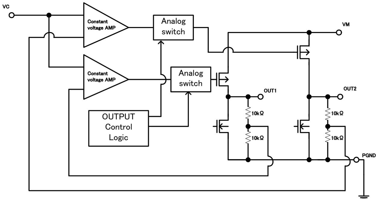
LV8075LP controls output voltage by controlling Pch power transistor to detect the voltage of OUT in order to obtain  $V_{OUT}$  voltage of  $V_C \times 2.0$ .
