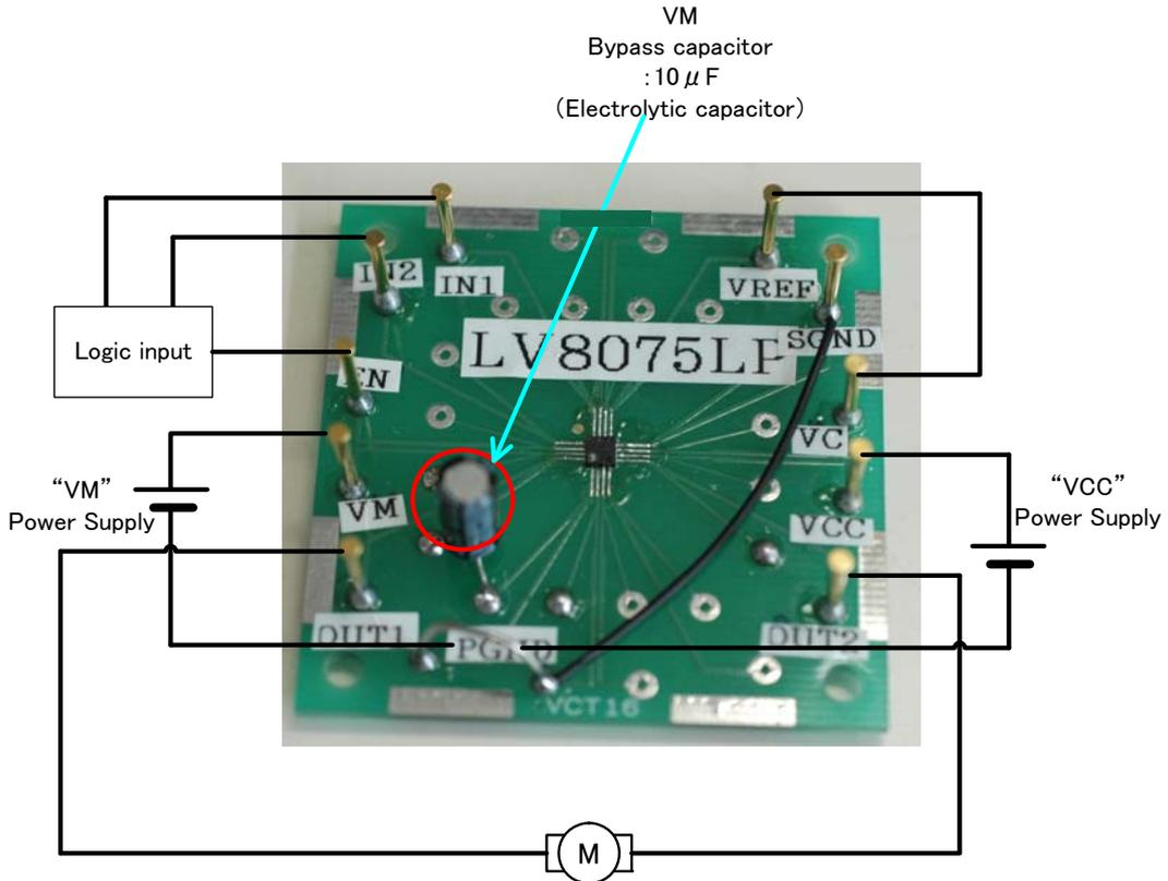
OUTPUT constant voltage 1.5V drive (VC voltage setting)
