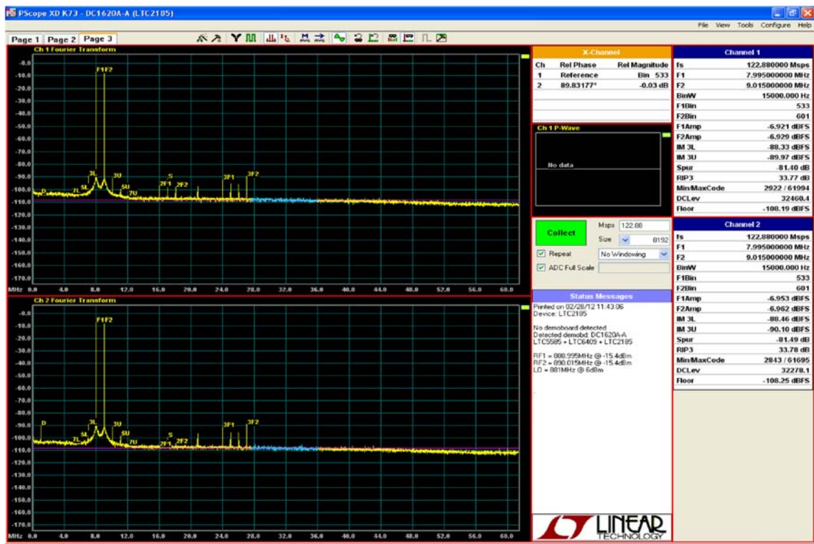
Figure 36. f_{RF} = 889MHz and 890MHz 2-Tone Receiver Test, f_{LO} = 881MHz. Ch.1 is the I Channel and Ch.2 is the Q Channel. Tested without LNA
