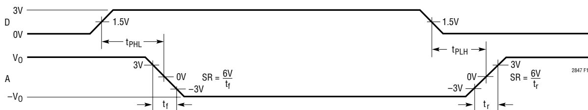
Figure 15. V.28 Driver Propagation Delays
