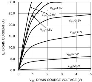
V<sub>DS</sub>, DRAIN-SOURCE VOLTAGE (V) Figure 1. Typical Output Characteristic
