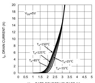
$V_{\rm GS},\, {\rm GATE}\text{-}{\rm SOURCE}\,\, {\rm VOLTAGE}\,\, ({\rm V})$  Figure 2. Typical Transfer Characteristic
