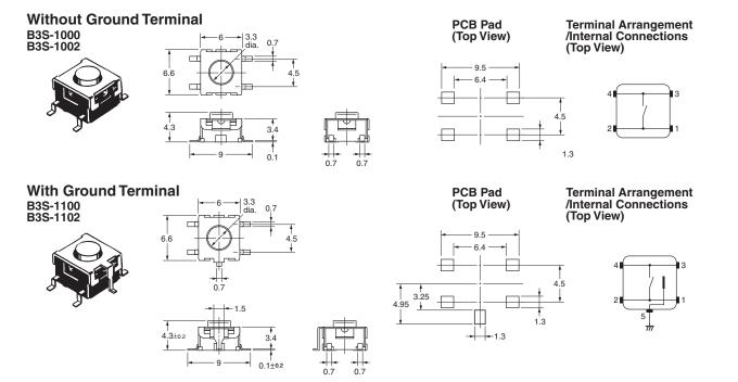
$\textbf{Note:} \quad \text{Unless otherwise specified, a tolerance of $\pm 0.3$ mm applies to all dimensions. No terminal numbers are indicated on the Switches.}$
