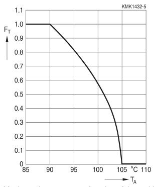
Maximum  $I_{RMS}$  current as function of the ambient temperature:  $I_{RMS}$  ( $T_A$ ) = Factor ×  $I_{RMS}$  (70 °C)
