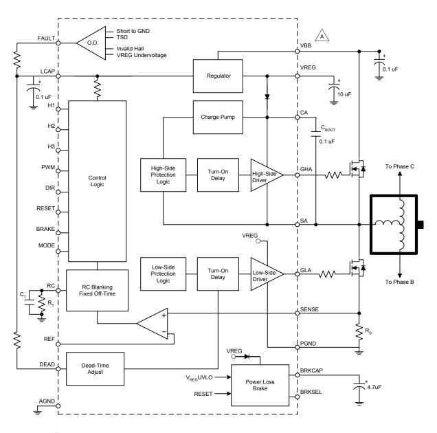
For 12 V applications, VBB must be shorted to VREG. For this condition, the absolute maximum rating of 15 V on VREG must be maintained to prevent damage to the A3938.
