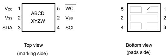
Figure 3. UDFPN5 (DFN5) package connections
