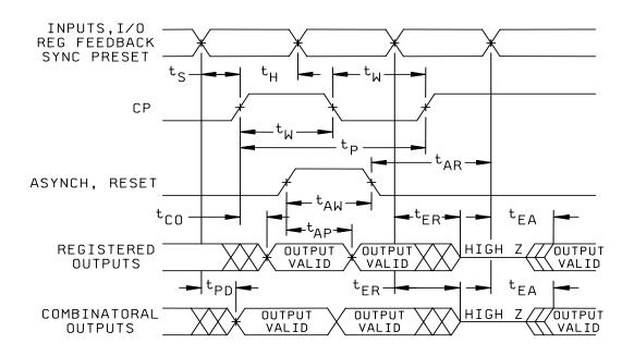
NOTE: Timing measurement reference is 1.5 V. Unless otherwise specified, input ac driving levels are 0.0 V and 3.0 V.
