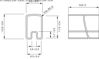
Tape and reel for SMT version 480 relays per reel, 2400 relays per box
