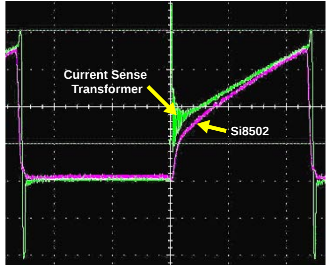
Figure 8. Leading-Edge Noise Suppression Waveforms (200 kHz, 9.3 A Load)
