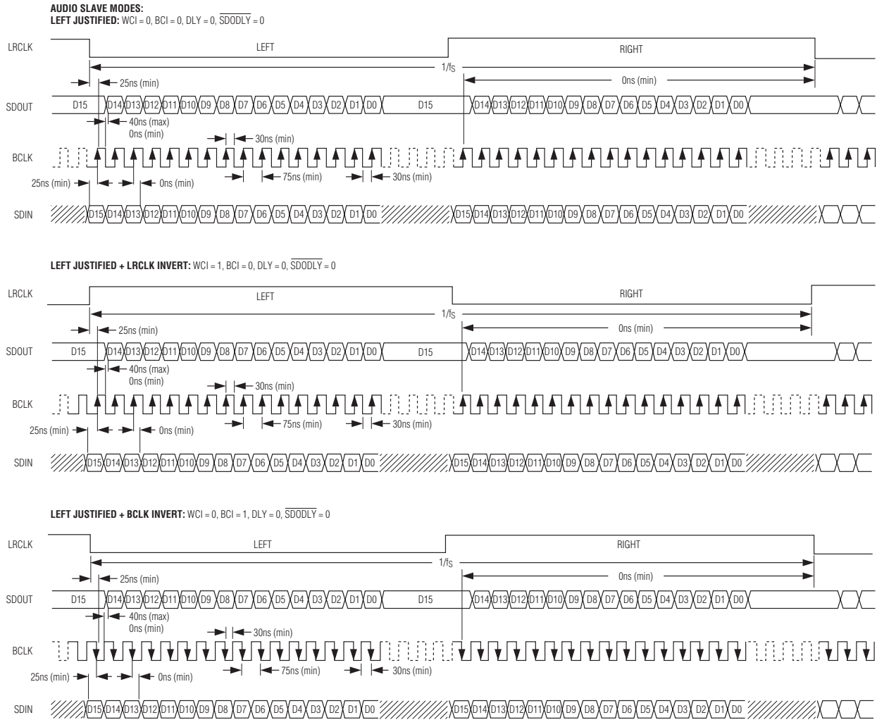
Figure 3. Digital Audio Interface Audio Slave Mode Examples (Sheet 1 of 2)
