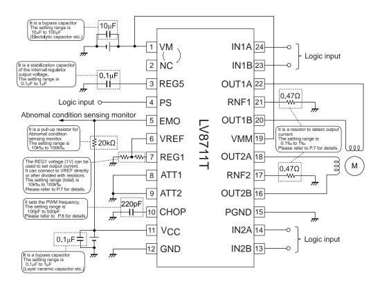
Each constant setting method for the above circuit diagram example is as follows:
