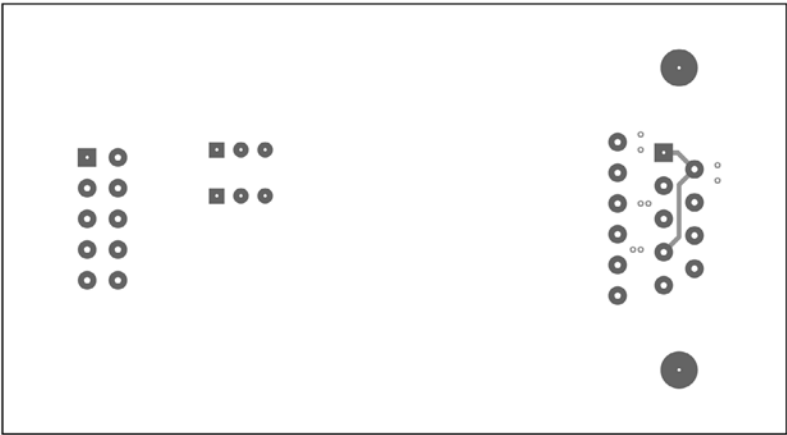
Figure 7d. Low EMI Demo Board Layout (DC1747A), Inner Layer 2
