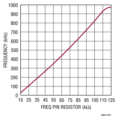
Figure 2. Switching Frequency vs Resistor on FREQ pin
