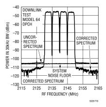
Figure 16: 4-Channel W-CDMA Spectrum
