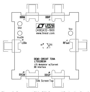
Figure 8. Component Side Silk Screen of Evaluation Board
