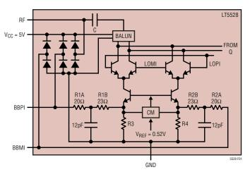
Figure 1. Simplified Circuit Schematic of the LT5528 (Only I-Half is Drawn)
