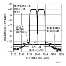
Figure 15: 2-Channel W-CDMA Spectrum
