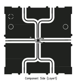
Figure 9. Component Side Layout of Evaluation Board
