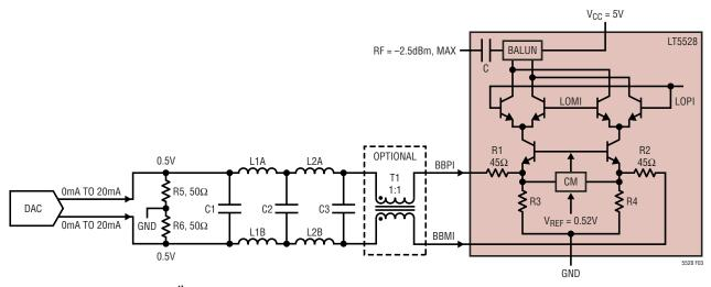
Figure 3. LT5528 5<sup>th</sup> Order Filtered Baseband Interface with Common DAC (Only I-Channel is Shown)
