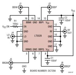
Figure 7. Evaluation Circuit Schematic
