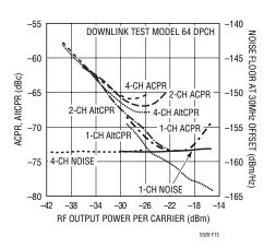
Figure 13: W-CDMA APCR, AltCPR and Noise vs RF Output Power at 2140MHz for 1, 2 and 4 Channels
