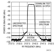
Figure 14: 1-Channel W-CDMA Spectrum
