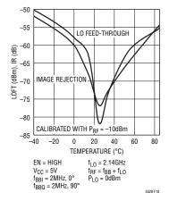
Figure 17: LO Feed-Through and Image Rejection vs Temperature after Calibration at 25°C
