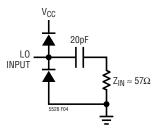
Figure 4. Equivalent Circuit Schematic of the LO Input
