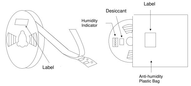
Tape and reel must be sealed with the anti-humidity plastic bag. The bag contains the desiccant and the humidity indicator.
