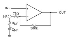
The voltage gain VG can be lowered by connecting an external resistor in series between the NF pin (pins 8 and 14) and  $C_{NF}$ .
