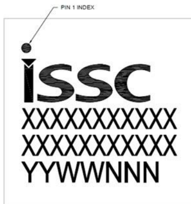
48 Lead QFN (6x6x0.9 mm)
