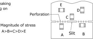
(3) The magnitude of mechanical stress applied to the Varistors when dividing the circuit board in descending order is as follows: push back < slit < V-groove < perforation. Also take into account the layout of the Varistors and the dividing/breaking method.
