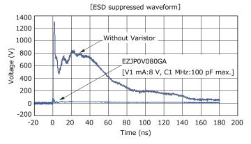
\*IEC61000-4-2 ··· International Standard of the ESD testing method (HBM) for electronic equipment ability to withstand ESD generated from a human body. It sets 4 levels of severity
