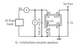
Figure 3) Test Circuit
