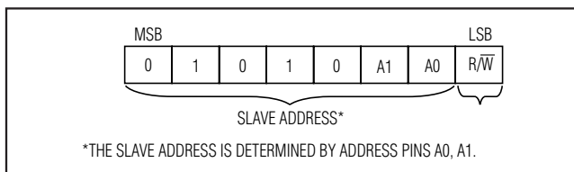
Figure 1. DS3502 Slave Address Byte
