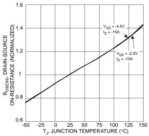
Figure 6 On-Resistance Variation with Temperature
