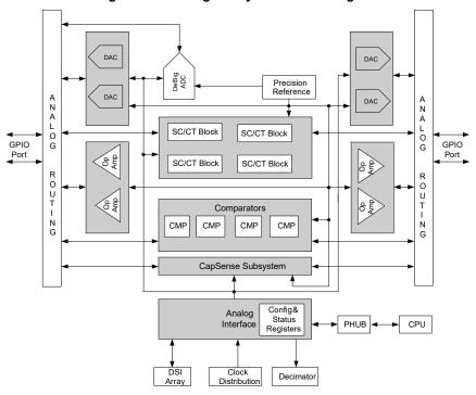
Figure 8-1. Analog Subsystem Block Diagram
