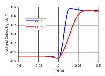
Figure 11-32. Opamp Step Response, Falling
