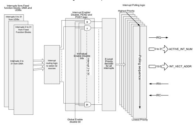
Figure 4-3. Interrupt Structure
