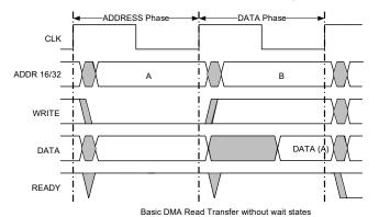
Figure 4-1. DMA Timing Diagram
