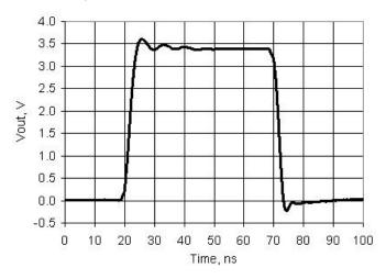
Figure 11-21. SIO Output Rise and Fall Times, Slow Strong Mode,  $V_{\rm DDIO}$  = 3.3 V, 25 pF Load
