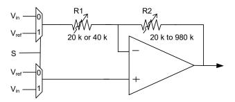
The PGA is used in applications where the input signal may not be large enough to achieve the desired resolution in the ADC, or dynamic range of another SC/CT block such as a mixer. The gain is adjustable at runtime, including changing the gain of the PGA prior to each ADC sample.
