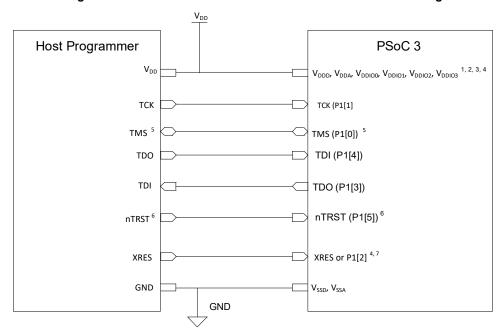
Figure 9-1. JTAG Interface Connections between PSoC 3 and Programmer
