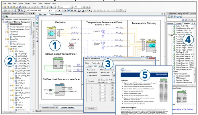
Figure 1. Multiple-Sensor Example Project in PSoC Creator
