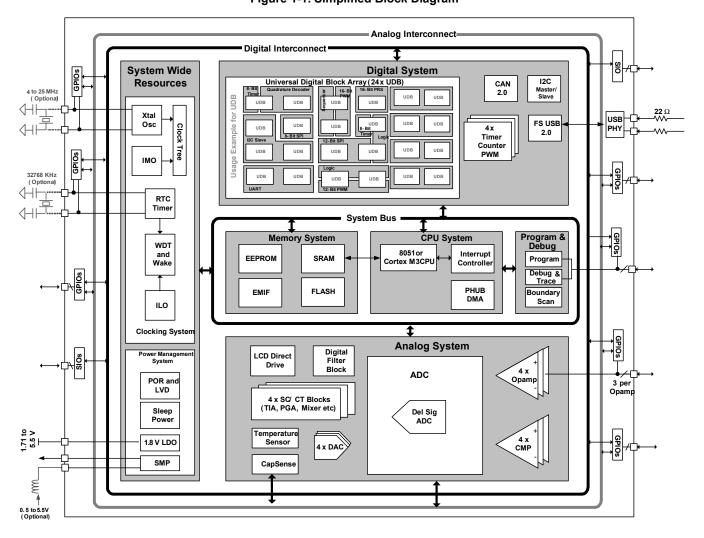
Figure 1-1. Simplified Block Diagram
