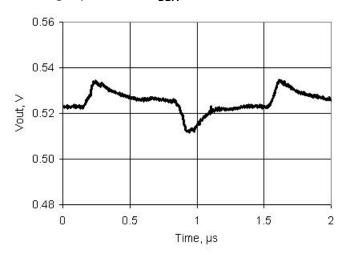
Figure 11-61. VDAC Voltage Noise, 1 V Mode, High speed mode,  $V_{\rm DDA}$  = 5 V
