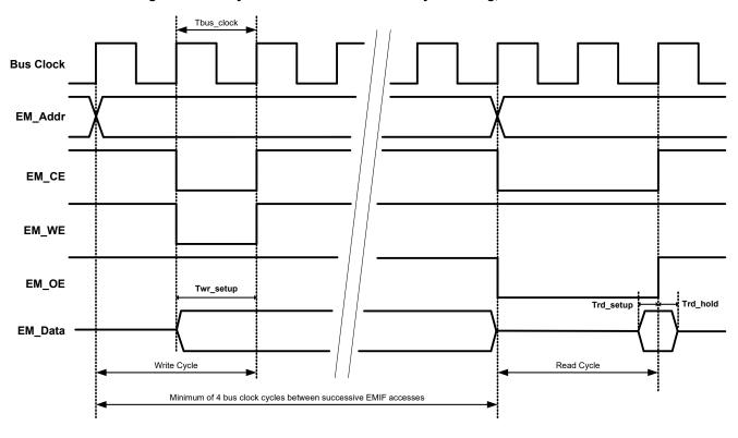
Table 11-63. Asynchronous Write and Read Timing Specifications<sup>[68]</sup>
