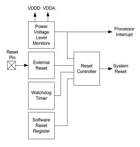
The term **device reset** indicates that the processor as well as analog and digital peripherals and registers are reset.
