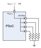
Conversely, for the 100-pin and 68-pin devices, the set of I/O pins associated with any VDDIO may sink up to 100 mA total, as shown in Figure 2-2.
