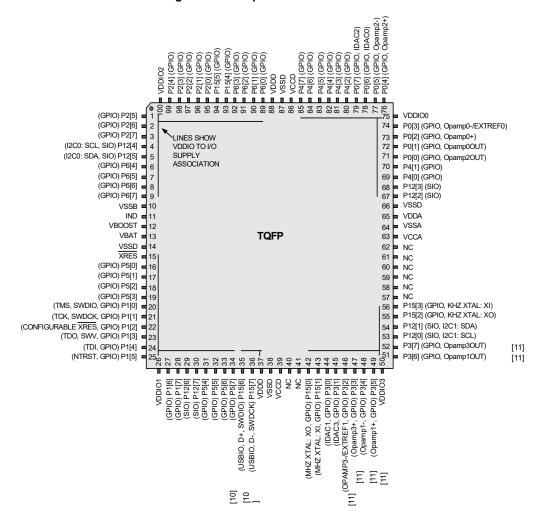
Figure 2-6. 100-pin TQFP Part Pinout
