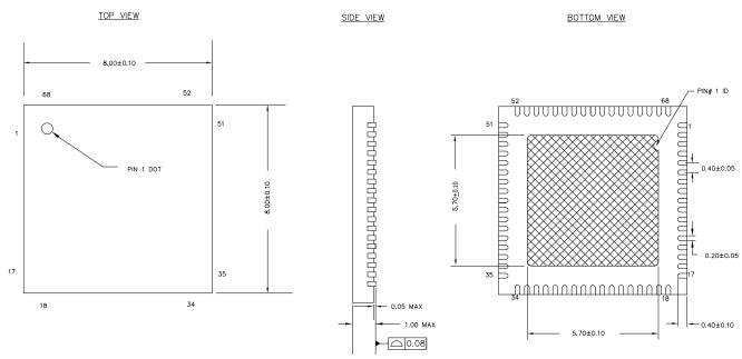
Figure 13-3. 68-pin QFN 8×8 with 0.4 mm Pitch Package Outline (Sawn Version)
