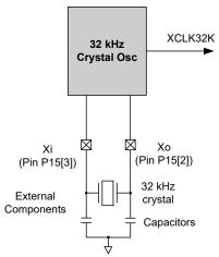
It is recommended that the external 32.768-kHz watch crystal have a load capacitance (CL) of 6 pF or 12.5 pF. Check the crystal manufacturer's datasheet. The two external capacitors, CL1 and CL2, are typically of the same value, and their total capacitance, CL1CL2 / (CL1 + CL2), including pin and trace capacitance, should equal the crystal CL value. For more information, refer to application note AN54439: PSoC 3 and
