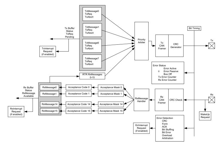
Figure 7-15. CAN Controller Block Diagram
