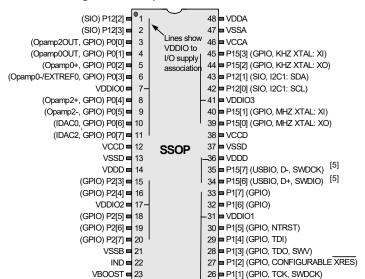
Figure 2-3. 48-pin SSOP Part Pinout
