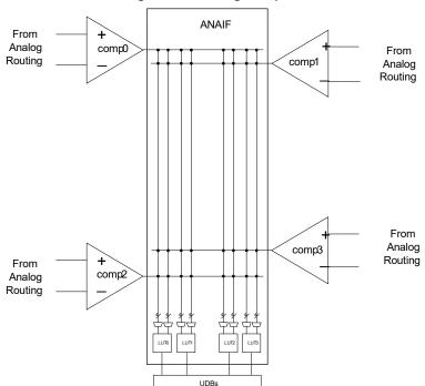
Figure 8-5. Analog Comparator
