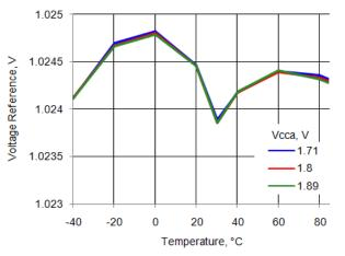
Figure 11-35. Voltage Reference Long-Term Drift
