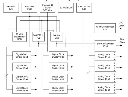
Figure 6-1. Clocking Subsystem
