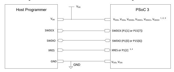
Figure 9-2. SWD Interface Connections between PSoC 3 and Programmer
