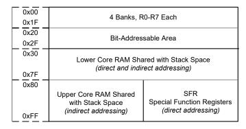
In addition to the register or bit address modes used with the lower 48 bytes, the lower 128 bytes can be accessed with direct or indirect addressing. With direct addressing mode, the upper 128 bytes map to the SFRs. With indirect addressing mode, the upper 128 bytes map to RAM. Stack operations use indirect addressing; the 8051 stack space is 256 bytes. See the "Addressing Modes" section on page 14.
