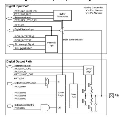
Figure 6-10. SIO Input/Output Block Diagram
