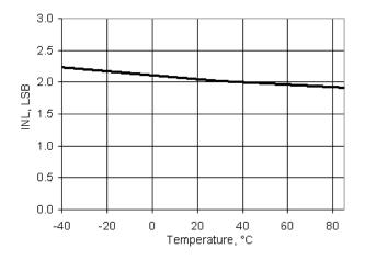
Figure 11-54. VDAC Full Scale Error vs Temperature, 1 V Mode
