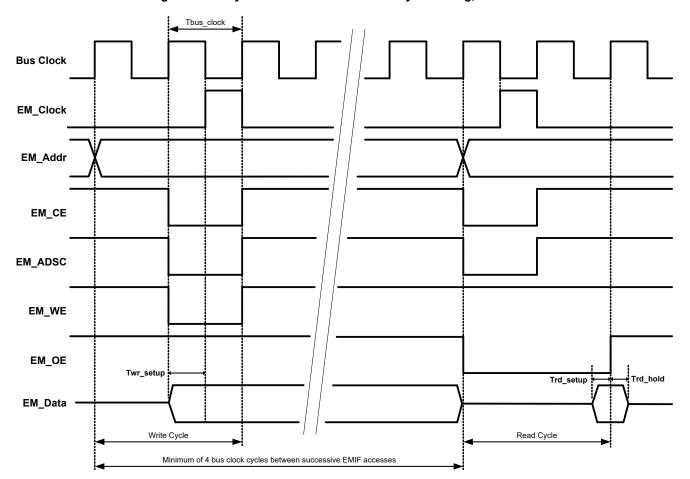
Figure 11-67. Synchronous Write and Read Cycle Timing, No Wait States
