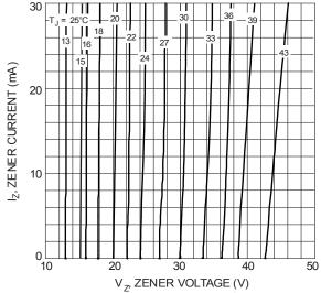
Figure 4 Typical Zener Breakdown Characteristics BZT585B13TQ - BZT585B43TQ
