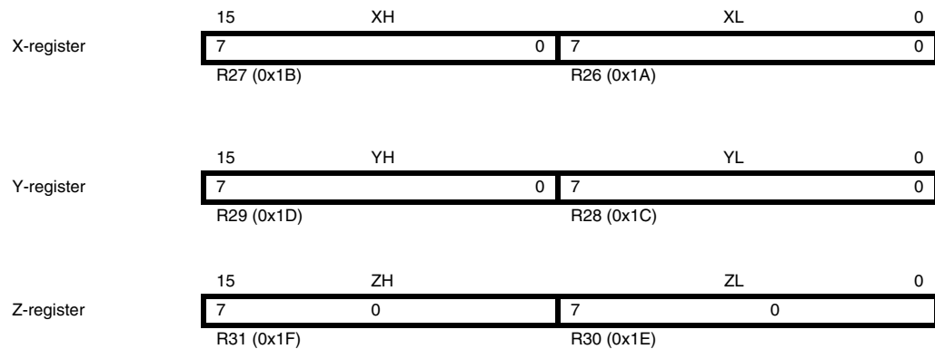
Figure 3-3. The X-register, Y-register, and Z-register.
