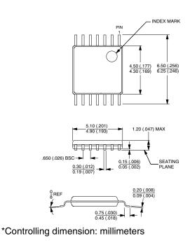
**20T**, 20-lead, 0.170" Wide, Thin Shrink Small Outline Package (TSSOP) Dimensions in (Inches) and Millimeters\*
