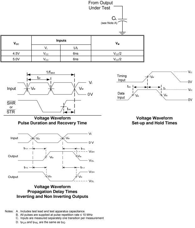
Figure 2. Load Circuit and Voltage Waveforms
