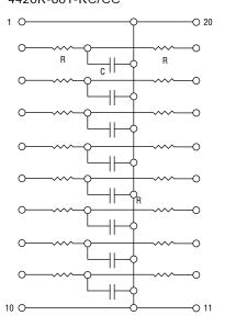
These low-pass filters are ideal for installation between I/O drivers and RS 232 connectors.
