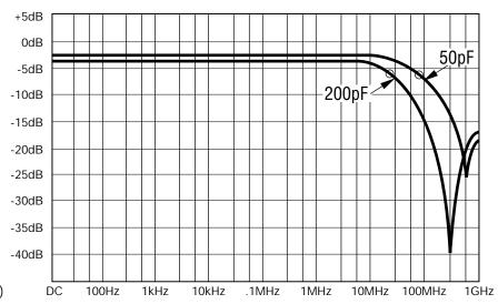
O indicates - 3dB rolloff frequency (f<sub>C</sub>)
