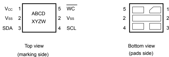
Figure 3. UDFPN5 (DFN5) package connections
