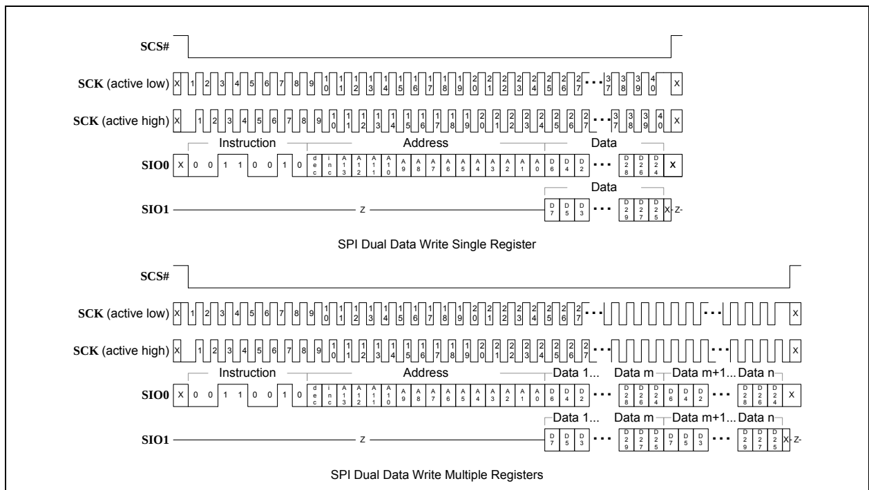
FIGURE 10-13: SPI DUAL DATA WRITE
