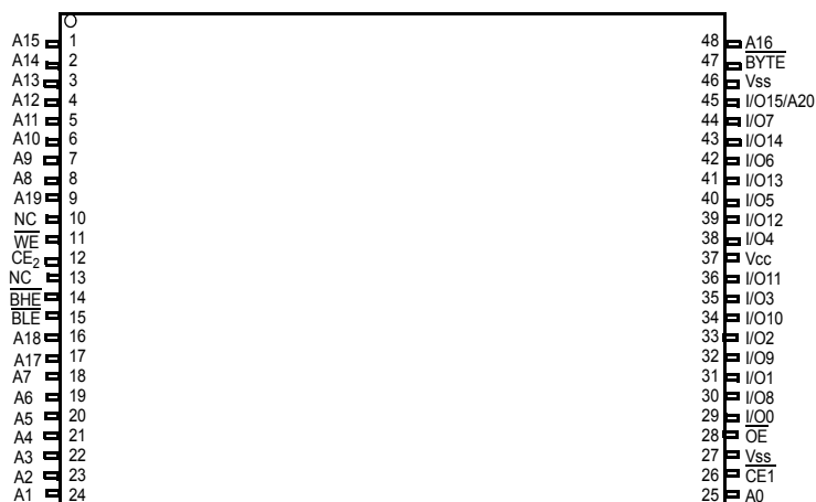
48-pin TSOP I pinout (Top View) [1, 2]
