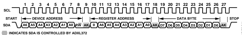
Figure 46. I 2 C Timing Diagram, Single Byte Write
