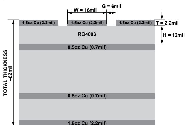
Figure 41. Probe Matrix Board Stackup
