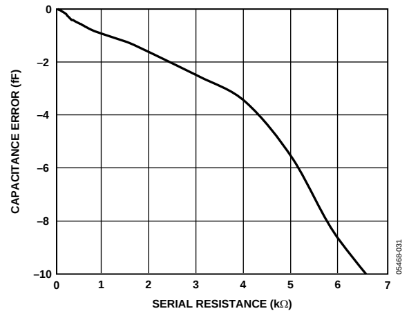
Figure 15. Capacitance Input Error vs. Serial Resistance, C_{IN}(+) to EXC = 21 pF, C_{IN}(-) to EXC = 23 pF, V_{DD} = 5 V, the Same Configuration as in Figure 34.
