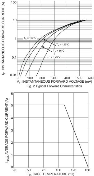
Fig. 4 Forward Current Derating Curve
