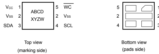
Figure 3. UFDFPN5 (DFN5) package connections
