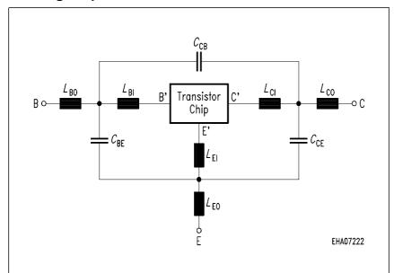
The TSFP-4 package has two emitter leads. To avoid high complexity of the package equivalent circuit, both lead are combined in on electrical connection.  $R_{\rm LxI}$  are series resistors for the inductance  $L_{\rm XI}$  and  $K_{\rm Xa-yb}$  are the coupling coefficients between the inductance  $L_{\rm Xa}$  and  $L_{\rm yb}$ . The referencepins for the couple ports are B, E, C, B´, E`, C´.
