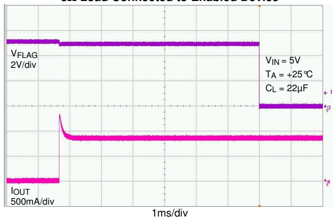
3Ω Load Connected to Enabled Device
