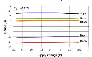
**Switch Points vs Supply Voltage**
