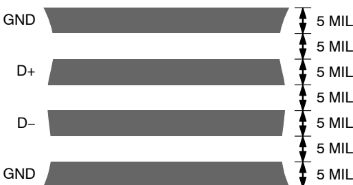
Figure 21. Typical Arrangement of Signal Tracks
