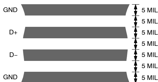
Figure 22. Typical Arrangement of Signal Tracks
