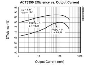
ACT6390 Efficiency vs. Output Current 95  $V_{IN} = 5V$  $V_{OUT} = 12V$ ACT6390-002 90 FREQ = G 85 Efficiency (%) L = 10µH 80 FREQ = IN L = 5.4µH 75 70 65 60 55 50 100 0 10 1000 Output Current (mA)
