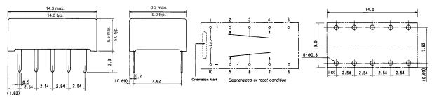
AL-D type (Double winding latching type)
