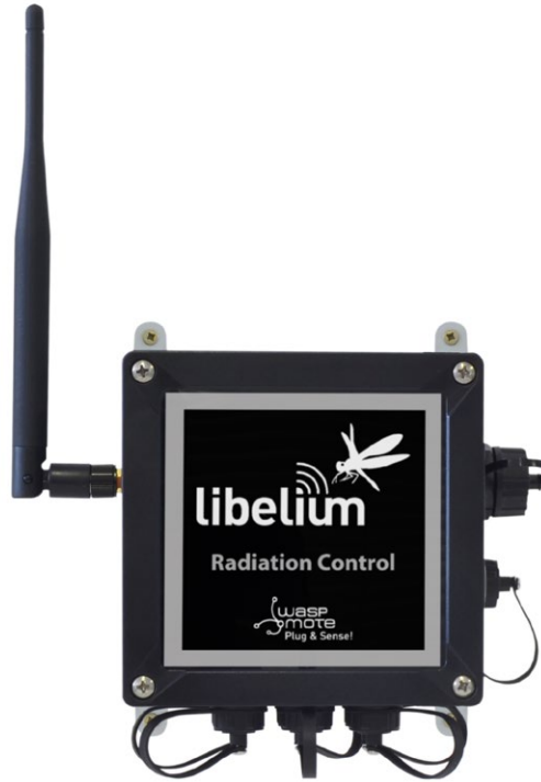
Figure 28: Radiation Control Waspote Plug & Sense! model
